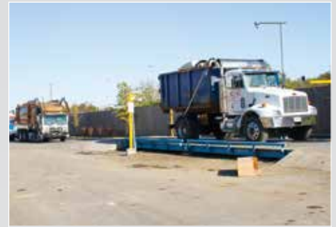
Each truck is weighed coming and going as the facility charges by the weight of materials received.
