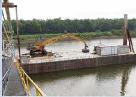
*Nearly all materials are barged to the facility and off loaded by a tethered excavator.*
