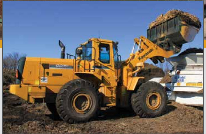
Kawasaki-KCM 90ZV loader charging the hopper of a Diamond Z1463B Grinder.
