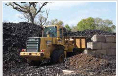
Kawasaki-KCM 60ZV 80 picking up Barclay material that will be loaded into the Granutech System or loaded into trucks to go directly into market.
