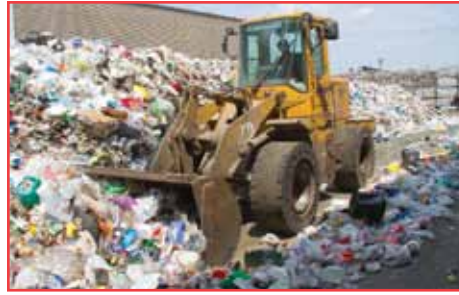
A Kawasaki-KCM 50ZV is used to push commingled recyclables into the processing plant for sorting.
