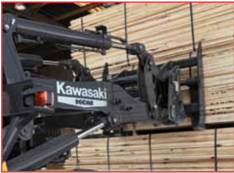
An industry-leading parallel linkage design provides a very good view of the forks for quick, smooth positioning for a quick pick.
