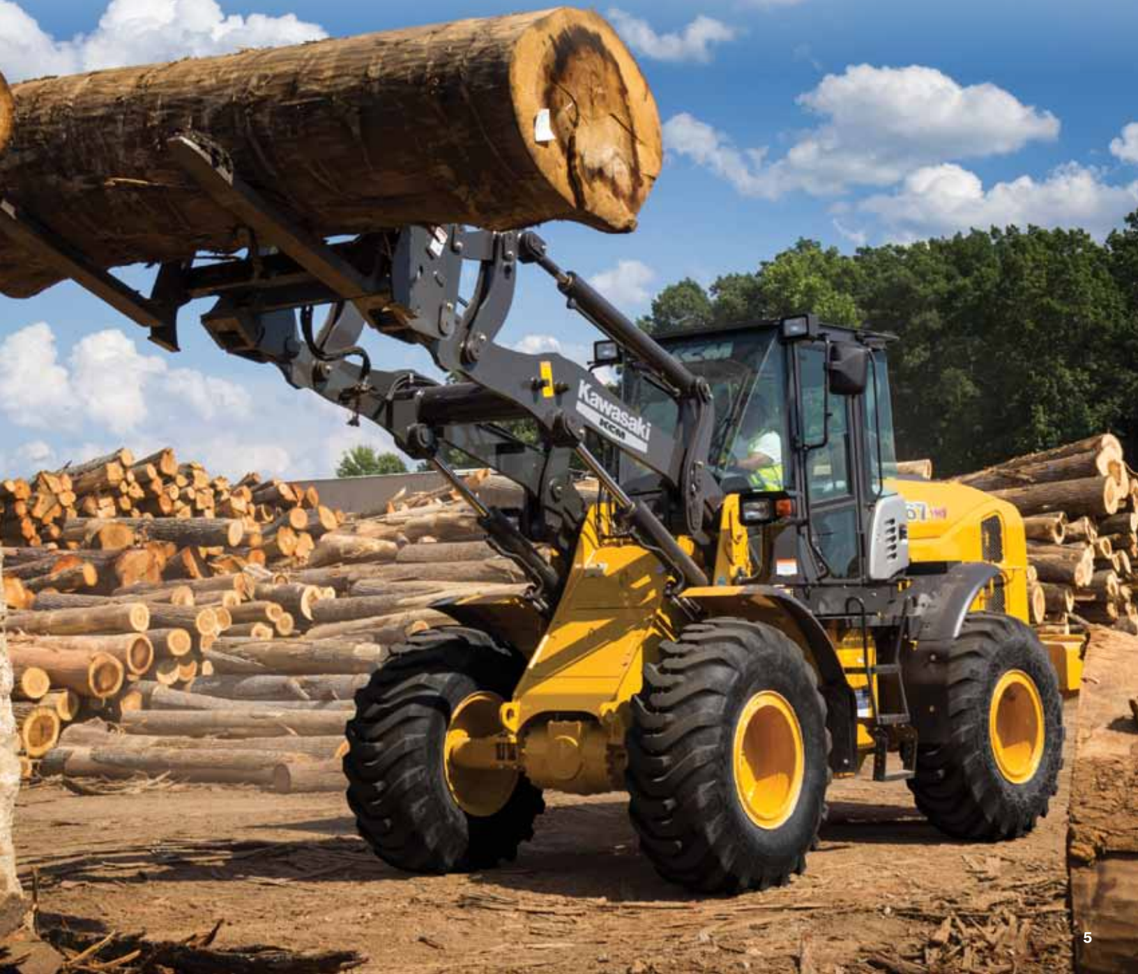
An industry-leading parallel linkage design provides a very good view of the forks for quick, smooth positioning for a quick pick.
