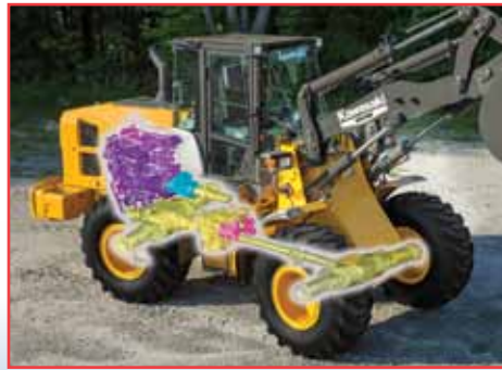
The open-center hydraulic operating system allows power to flow to the most pressing need.
