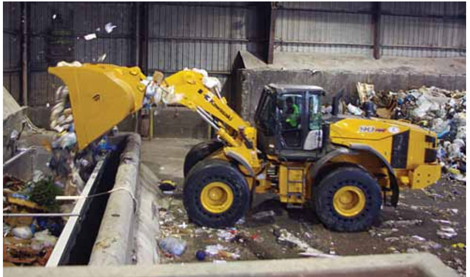
The 90Z7 loads refuse onto large trailers.
